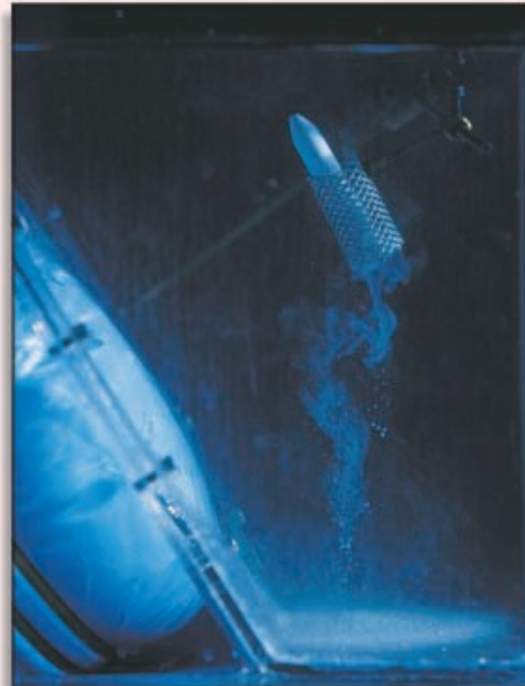
The chalk is being pulverized in the test pool by the Stonelith's shock waves
